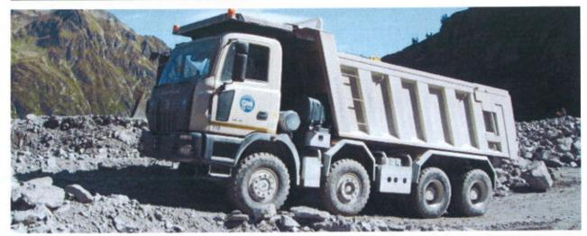
Groupement Marti Implenia has purchased 10 Astra HD8 trucks for the construction of a pumped-storage underground site of the Nant de Drance hydroelectric power plant. The installation is being built inside the mountain with an access tunnel of 5.6 km. The trucks are operating on demanding 12% steep slopes, powered by a 353 kW Iveco engine with an Allison automatic transmission spec'd for the application.
